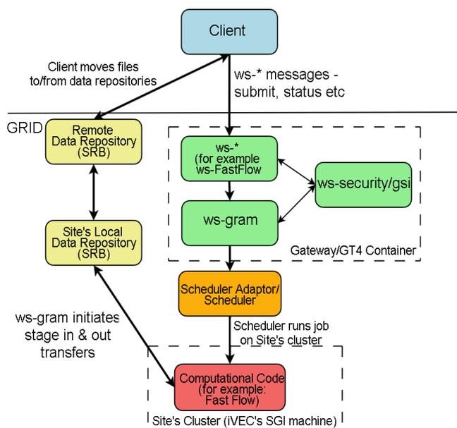
Figure 1. Geosciences Grid SOA architecture
