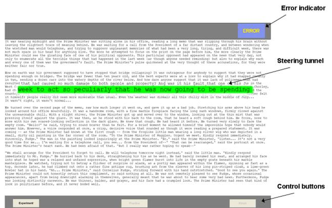
Figure 7: The interface for the second experiment, where participants were required to drag the cursor through the highlighted tunnel. The tunnel is represented by a green rectangle that covers a number of words, depending on the tunnel length.
