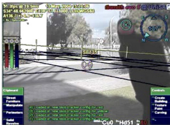
Figure 7 - Output from the Tinmith modelling software, showing the augmented reality overlay. The cursor representing the detected marker location is being drawn using values from the RC200.
