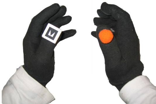
Figure 2 - Original ARToolkit marker shown attached to the left glove, and new robust ball-shaped coloured markers shown attached to right glove.
