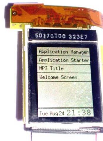
Figure 5. The task manager application running on the current watch prototype.
