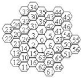
**Fig.7 A collection of  $7^2 = 49$  hexagons with labelled addresses**
