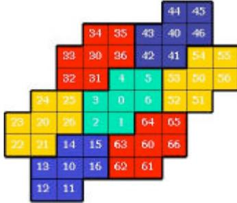
**Fig.10 the first 49 Pseudo pixels with labelled spiral addresses**
