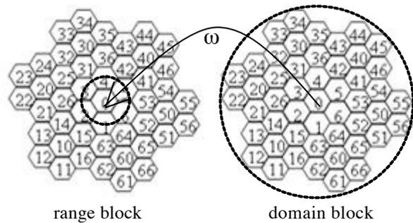
**Fig.12 Range and domain blocks in Spiral Architecture**
