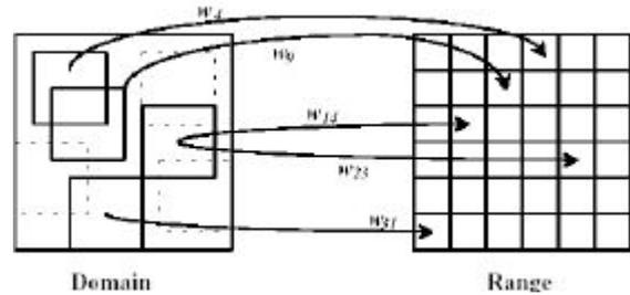
Fig. 3 Each range block is constructed by a transformed domain block
