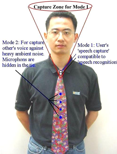
**Figure 2: Structure of proposed wearable microphone array embedded in a tie**
