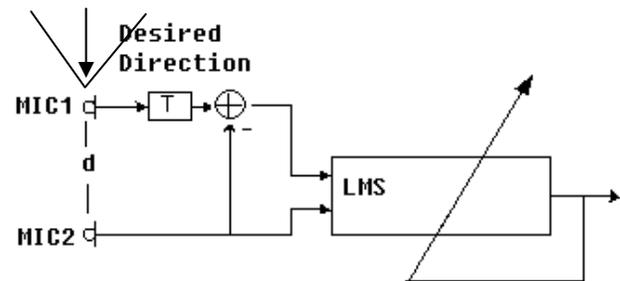
**Figure 3: Diagram of adaptive microphone array structure**
