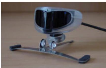
Figure 5: Infrared laser tracking device *Smart-Nav*.
