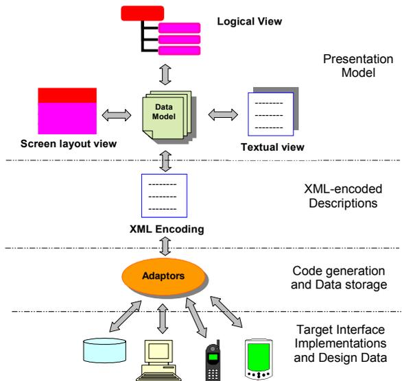
Figure 3. Adaptive GUI design tool architecture.
