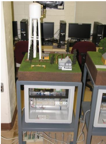
Figure 2: MSU SCADA Security Laboratory water tower application with view of SCADAPack programmable logic controller under cart.
