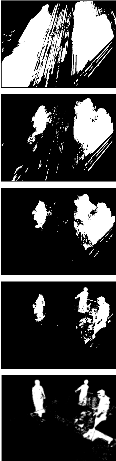
Figure 17: Results of progressive Shape-from-silhouette reconstruction with increasing number of cameras. From top to bottom: projection of the 3D reconstruction with 2, 3, 4 and 5 cameras. Bottom image: original (noisy) 2D foreground.
