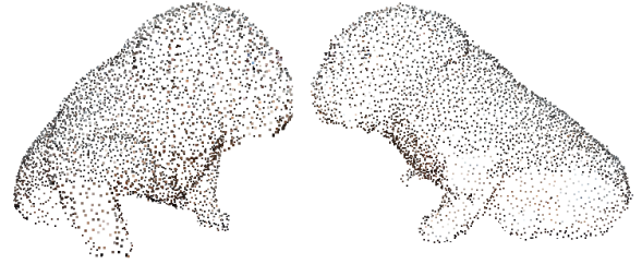
Figure 4: Additional 3D points generated by exploiting the silhouette information.
