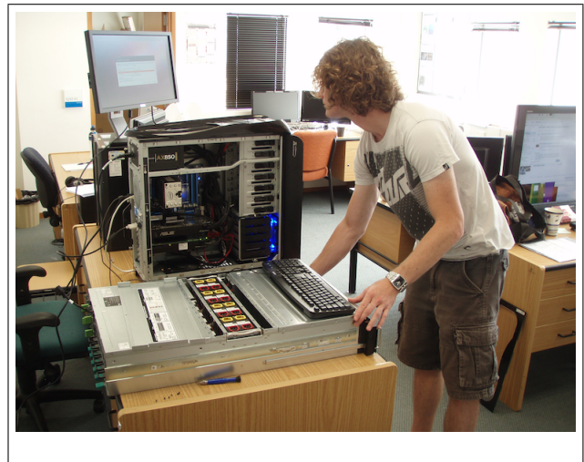
Figure 5: The Dell C410x Chassis - shown with cooling fans exposed, in process of having GPUs installed and HCI connector cables linking the extended PCI bus to the internal PCI bus of a hosting PC..
