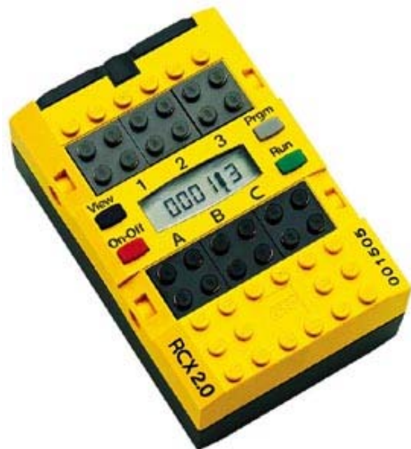
Figure 1: The RCX brick (Devine 2008). The input ports (1, 2, 3) and output ports (A, B, C) have electrical connections in the otherwise normal Lego ‘bumps’.
