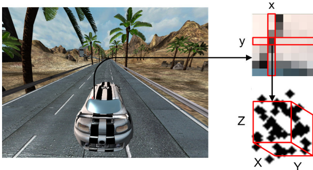
Figure 6: Relationship between a fragment in screen space and the related region of the vector (\mathbf{R}, \mathbf{C}) . The cube in object space is the equivalent region of the fragment at screen position (x, y) . The number of points p in the cube corresponds to the number of points in the model test frame at (x, y) .
