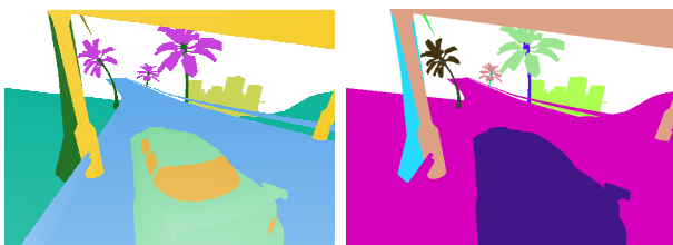
Figure 5: Example of object map (left) and matrix map (right) of a frame. Colours identify different objects in the object map and different world-view-projection matrices in the matrix map. The depth buffer is encoded by the \alpha channel of the object map.
